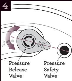
Ensure Pressure Regulator/Release Valve is turned to Pressure position shown.
